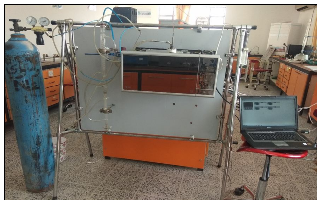
Fig. 2: Microwave pyrolysis process unit.
